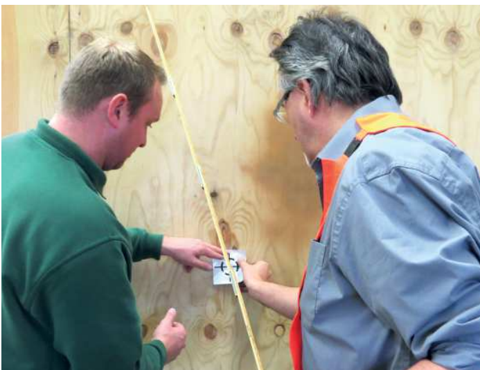
5. Marking of the three-dimensional centre of gravity on the package: The three-dimensional centre of gravity is captured! A Marking identifies the position of the three-dimensional centre of gravity. Now the freight could be secured and transported.
