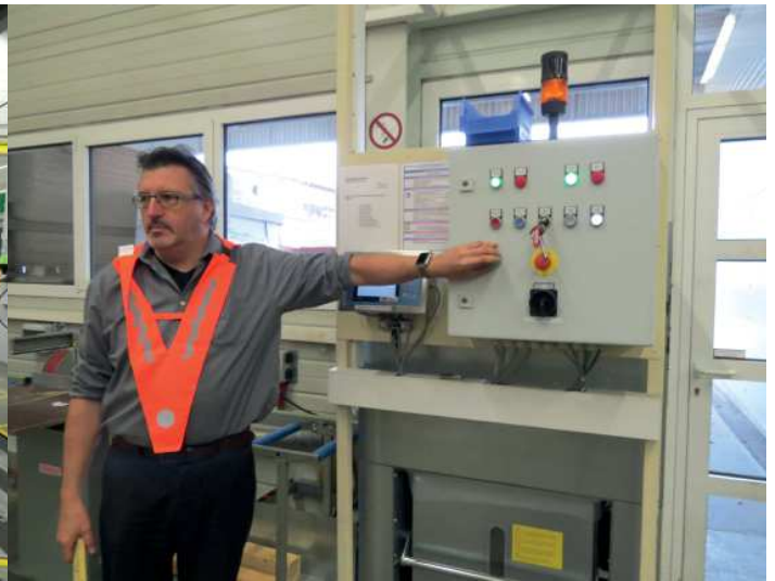
2. Touch of a button starts the three-dimensional measurement: A touch of a button on the weighing terminal starts the automatic measurement of the three-dimensional centre of gravity. The long side of the weighing bridge lifts and tilts itself. The package follows the movement.
