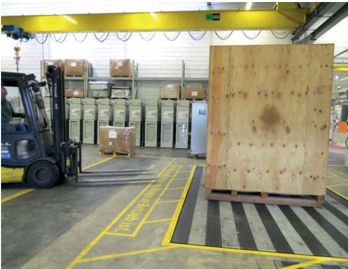
1. Determination of the centre of an area: The package is put on the weighbridge.. Its content has an eccentric centre of gravity. The 3D 5000 measures up the centre of an area automatically.
