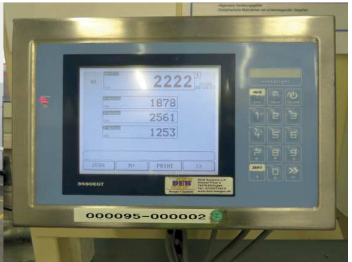
4. Calculation of the three-dimensional centre of gravity: The balance calculates the three-dimensional centre of gravity with the help of both centres of an area and with the degree with which the weighing bridge tilts. After a few seconds the display shows the coordinates of the three-dimensional centre of gravity - the length, the wide and the amount.
