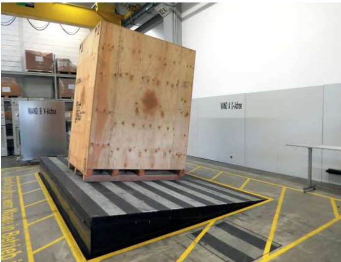
3. Calculation the centre of an area in inclined position: Due to the inclined position the centre of an area shifts. The 3D 5000 measures up the centre of an area once again - this time in inclined position. Now the balance has captured all values for the calculation of the three-dimensional centre of gravity.
