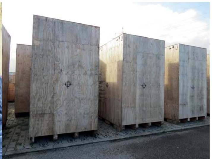
6. Packaged and provided with centre-of-gravity-markings - medium-voltage systems ready for transport. The freight has its drawbacks. The shapes of the medium-voltage systems are complex and far away from each standard.
